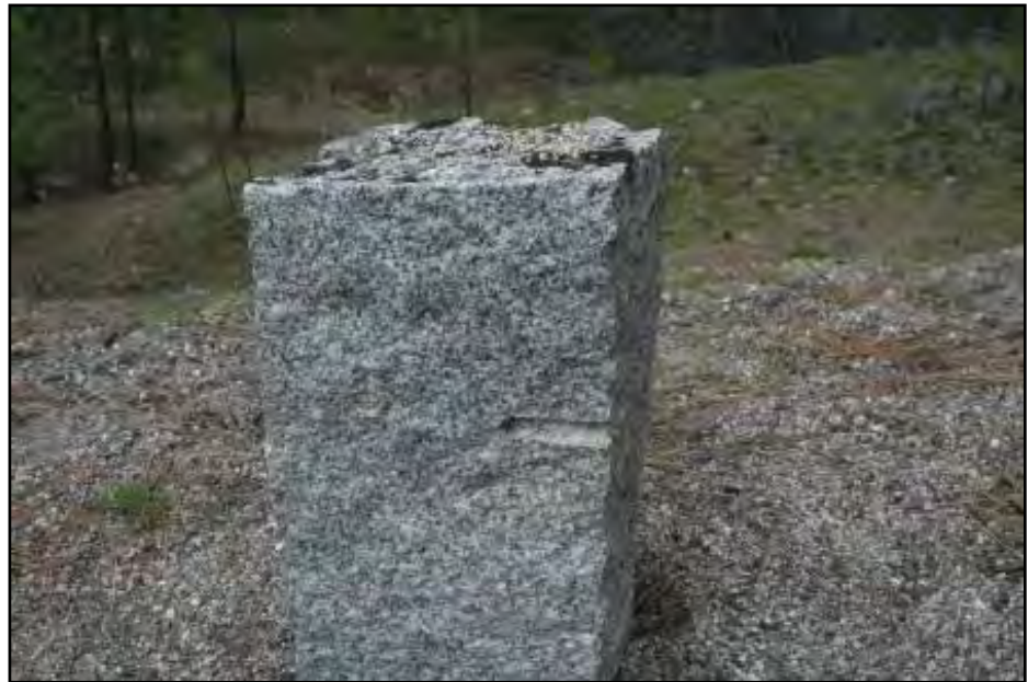
Figure 9: Granite split with feather and wedge method, Rutter Parkway, Spokane
